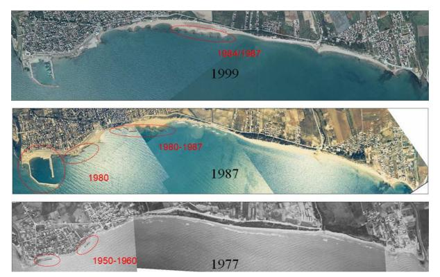
**Figure 2**: shoreline changing between 1977 and 1999. All the breakwaters in front of the second and the third beach, were built after the harbour construction.
